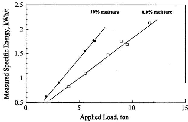
Fig. 7. Effect of applied load on the specific energy consumption at 0 and 10% feed moisture
