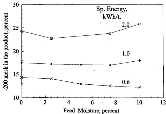
Fig. 10. Effect of feed moisture on the production of fines, -200 mesh
