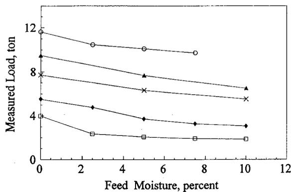
Fig. 2. Effect of feed moisture on the applied load at various load levels.
