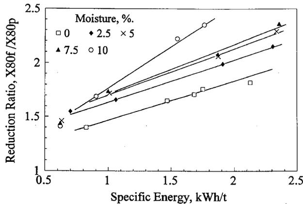
Fig. 14. The reduction ratio, X80f/X80p, as a function of specific energy consumption
